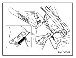
The lever that allows you to tilt the steering wheel is located under the steering column.
